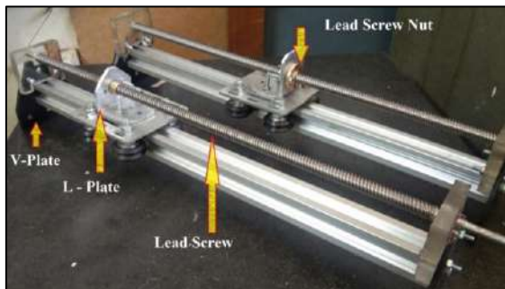
Figure 14 V-slot gantry system manufactured in PIEAS
